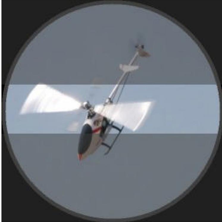
The Main rotor blades appear to stop when the shutter speed matches the Rotor RPM
