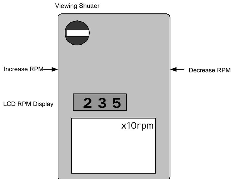
The tach automatically shuts off after 30 seconds of inactivity. It will remember the last set RPM. After wakeup, allow 3 seconds for the shutter RPM to stabilize.
